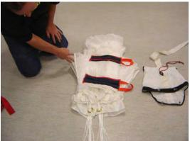
S fold the nose under the canopy as shown to the width of the remainder of the canopy.
