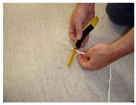
5. Pass the lower part of the toggle through the loop at the end of the control line.
