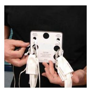
At the factory, the links are assembled onto a card identifying each link and steering line. This is to be used as a guide only. It is the responsibility of the assembling/inspecting rigger to verify that each link is connected to the proper riser and each steering line is connected to the proper steering toggle. Before securing the links fully, check line continuity. Ensure that each line group passes through the correct slider grommet and there are no twists, tangles, or knots in the lines.
