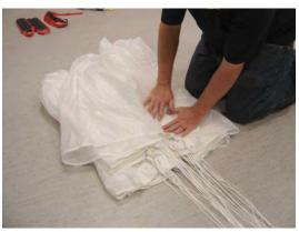
Upon finishing the flaking of the canopy, verify that the tail is evenly split so that the center seam of the center cell runs up the middle of the top of the pack job.
