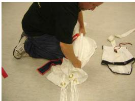
At this point, three cells of the nose should extend from each side of the pack job. Count the cells at the nose and verify that the previous step did not pass any fabric around any portion of the nose of the canopy.
