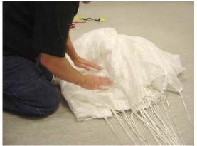
Neatly flake the tail of the canopy, grouping the steering lines in the middle and making folds of material to each side, maintaining a constant width for each fold.
