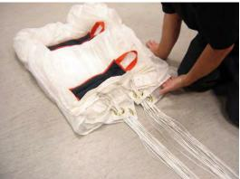
The following section gives general guidelines for folding the canopy to fit into a freebag. Because of the variation in size and shape of container systems, freebags from different container manufacturers will, of necessity, vary in shape and size. The exact amount of material in each fold of the canopy will then have to vary so that the material is distributed to fit in the freebag and container being used.
