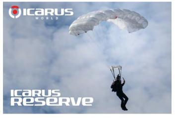
The suspension lines are 725lb Spectra, with the lower steering lines made of 1000lb Spectra. Line attachment points are secured with double bartacks for higher strength. *ICARUS WORLD Reserve* Spectra lines are coated to assure better protection during packing, opening and after landing, better resisting damage from bushes, sand, Velcro hook, etc....
