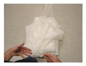
Now, precisely neaten the folds of the canopy. For each grouping of lines, count and verify that all lines are neatly grouped in middle and the A-B, B-C, and C-D folds are neatly and precisely folded to each side.
