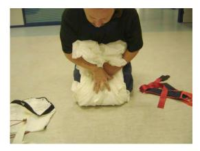
Then carefully make a second S fold as necessary to form the canopy into the proper shape to fit in the freebag.
