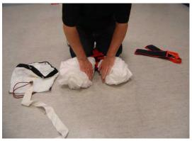
The ears of the molar pack job may need to be reduced in length to fit in the freebag. This can be accomplished by folding or compressing the ears to achieve a uniform distribution of fabric in the freebag. The end result is a canopy, neatly folded, distributed evenly, and formed into a shape that can be placed into a freebag according to the container manufacturer's instructions.
