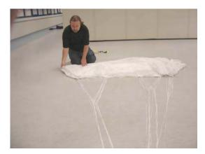
The nose of the canopy should be split so that 3 cells are arranged to each side and the middle cell is spread open. When arranging the canopy over the shoulder, the nose should face the rigger. When the canopy is on the floor, the nose should face the floor.
