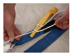
4. S fold the excess control line. Secure the toggle and excess control line according to the instructions of the harness manufacturer.
