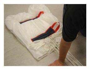
Now, pull the slider all the way up to the canopy, placing it symmetrically against all four slider stops. Flake the slider to each side between the line groups and neatly organize the fabric.
