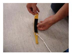
6. Pull all excess line through the toggle until the loop is taut.
