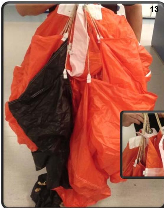
Since all the lines are bunched up in the middle, pull each stabilizer panel out one by one until they form an irregular shape and be sure that none of the lines are wrapped around a slider stop on a stabilizer.
