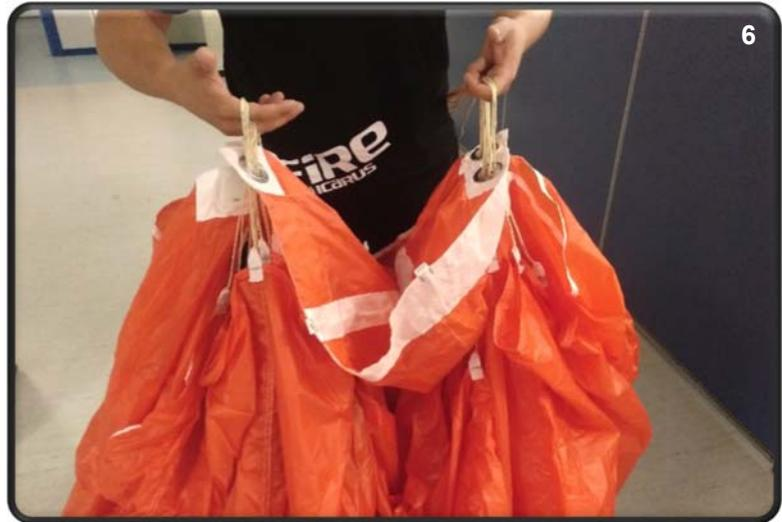
The tail should be farthest from the rig and the nose openings should be facing the rig. If the reverse is true and the rig is positioned correctly as described earlier, then the parachute was attached to the harness backwards! If you do not know how to solve this problem, get qualified assistance from a FAA rated rigger / instructor or a proper rated equivalent of your country.
