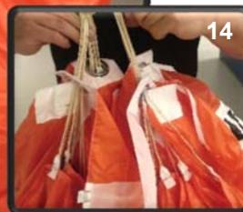
Now take the last fold of the stabilizer and fold it towards the center till the slider, so the lines also the steering lines will be covered like in the picture 15.
