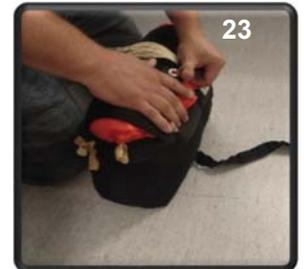
It takes practice to pack quickly and neatly. Every jumper has his own technique to make this easier and you'll quickly develop your own. The whole canopy should be in the bag before you follow your rig manufacturer's instructions for closing the bag, stowing the lines, placing it in the pack tray, and closing container.
