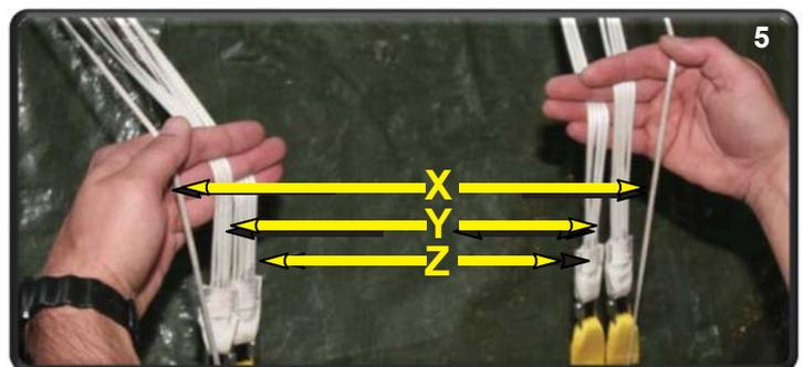
Start moving up the lines, allowing them to slide between your fingers while pushing the slider ahead until you reach the bottom of the parachute. While doing this make sure that the steering lines and the lines of front and rear riser groups run free and are not entangled with each other. When you reach the parachute, pull both hands apart approximately the width of the slider. Shake the parachute a few times to settle everything.
