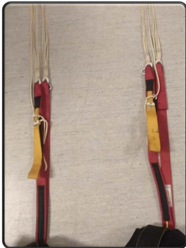
Set the deployment brakes according to the manufacturer instruction of your harness container system or riser manufacturer.
